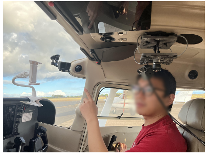
Fig. 11: Setting up the shock-absorbing fixture for the cockpit camera in a Cessna 172S. © Mahdi Al-Hussein 2023
